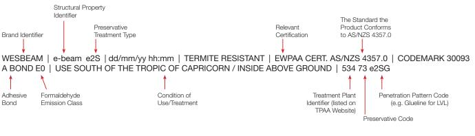
To be compliant with AS/NZS 4357.0, each piece of LVL must have the following information labelled on it:
